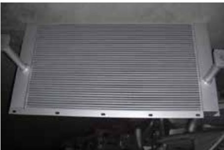
External oil-cooler for compressor
